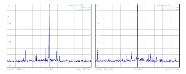
Fig. 2: Spectra of the transmitted signal amplitude in units of [dB] at 3 kHz bandwidth as function of the frequency offset when using mode CW for the setup of transceiver K3, transverter TR144H+40, and power amplifier BEKO HLV-600. The system power output has been about 400 W (left) and 550 W (right).
