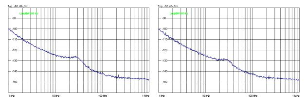
Fig. 1: Phase noise in units of [dBc/Hz] as function of the frequency offset for the setup of transceiver K3, transverter TR144H+40, and power amplifier BEKO HLV-600. The system power output has been about 400 W (left) and 550 W (right).
