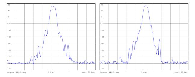
Fig. 3: Spectra of the transmitted signal amplitude in units of [dB]at 3 kHz bandwidth as function of the frequency offset when using mode SSB for the setup of transceiver K3, transverter TR144H+40, and power amplifier BEKO HLV-600. The system power output has been about 400 W (left) and 550 W (right).
